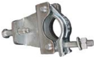
Fix Girder Coupler & Swivel Girder Size: 48.3 mm (EN-74) Provides a rotating coupling of a scaffold tube to an I' beam girder. Must be used in pairs.
