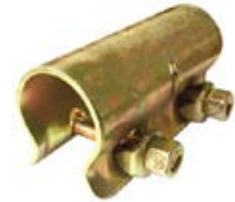
Sleeve Coupler Size: 48.3mm (EN-74) Used as the external connection of 2 tubes end-to-end provides a more secure joint than the Joint Pin.
