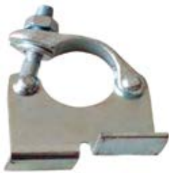
Board Retaining Coupler Size: 48.3 mm (EN-74) Boards are quickly locked in the correct position, providing high resistance to both lateral & upward movement.
