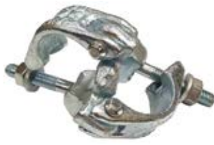
Double Coupler Size: 48.3mm (EN-74B), Used to join 2 scaffold tubes at a right angle (90°).
