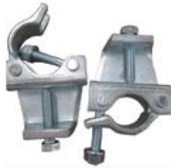
Girder Coupler Fixed Size: 48.3 mm (EN-74) Provides a fixed 90° coupling of a scaffold girder. Must be used in pairs.
